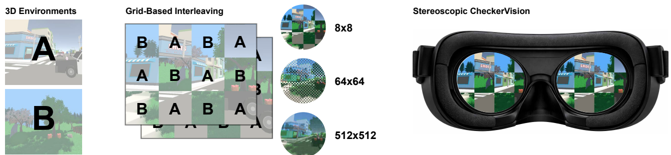
Figure 1: CHECKERVISION uses a checkerboard segmentation pattern to interleave two virtual environments (A/B) across the entire field of view while preserving stereoscopic depth perception. We implemented three grid resolutions: coarse (8×8), medium (64×64), and fine (512×512).
